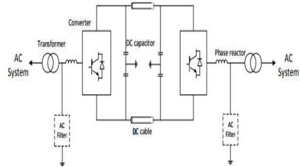
Fig 3 VSC-HVDC Components
