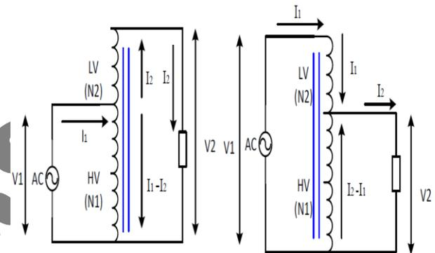
Fig 4 Autotransformer is boost (left) and buck (right) operation
